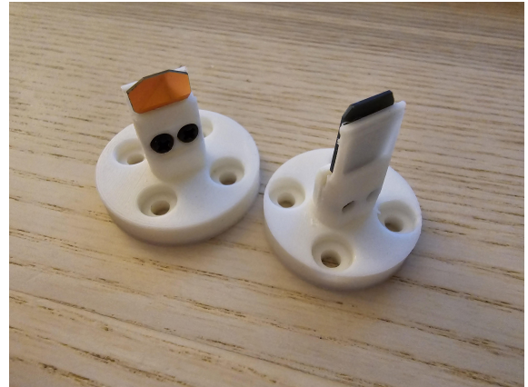
Figure 5. The fixture of the mirrors
